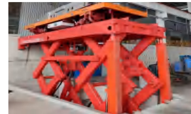
固定剪叉升降平台带防坠推杆 + 机械硬支撑双保险 Fixed scissor lift platform with anti-fall push rod and mechanical hard support double insurance
