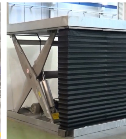
不锈钢剪叉式升降机加风琴罩防护 Stainless steel scissor lift with organ cover protection
