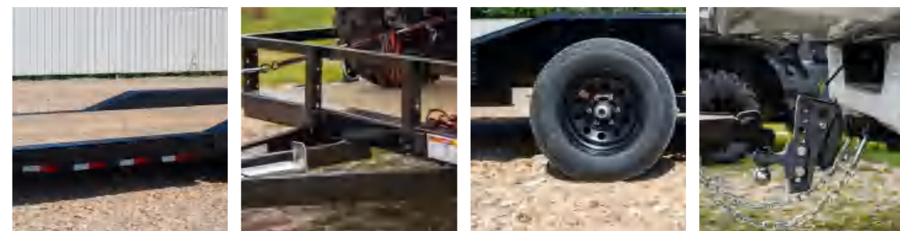
标准支柱孔 Standard stake pockets | 侧面可拆卸 Removable Sides | 前轮自动调节制动 Forward self-adjusting brakes | 锁扣联接器 Latch Coupler
