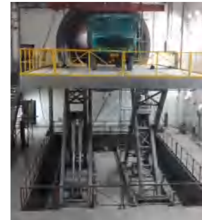
飞机风洞实验检修升降平台 Aircraft wind tunnel test maintenance lifting platform
