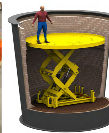
钢铁行业重型钢包升降器 Heavy Duty Ladle Lift for Steel Industry
