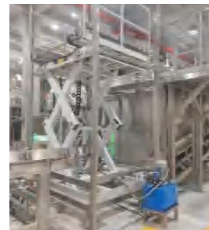
316 不锈钢酒庄固定剪叉升降平台 316 stainless steel winery fixed shear and lifting platform
