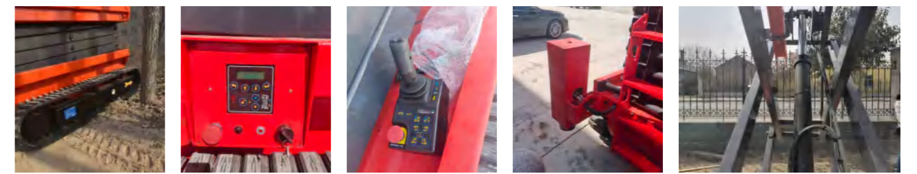
履带细节 Track Detail 控制面板 control panel 操作杆 joystick 支腿 outrigger 液压缸 Hydraulic Cylinder
