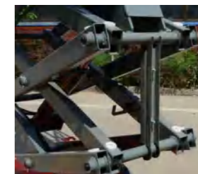
维修支杆 Maintenance support rod
