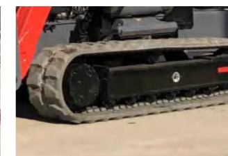
无痕橡胶履带 Non-marking rubber tracks
