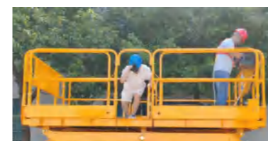
双向延伸台面 Bidirectional extension tabletop
