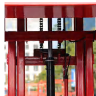
加粗板式链条 Thick leaf chain
