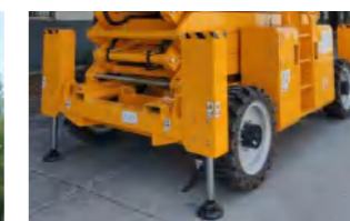
自动调平液压支腿 Automatic leveling hydraulic support legs
