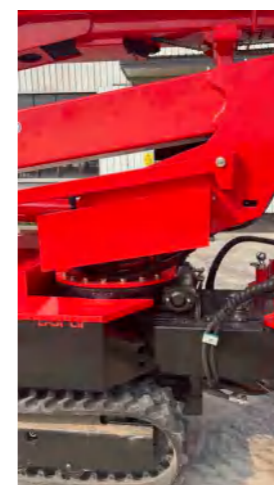
履带整机旋转可 360 度 The whole machine can rotate 360 degrees
