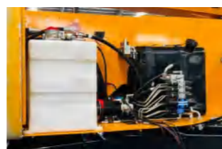
液压油箱 Hydraulic oil tank
