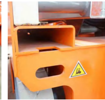
叉车孔吊装孔 Forklift hole Lifting hole
