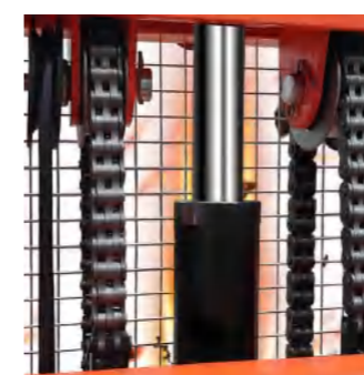
加粗板式链条 Heavy plate chain
